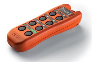
EVO is a brand new radio remote control, developed and produced by ELCA in full compliance with applicable laws\* for machines and industrial lifting and handling. It consists of 6 double step push buttons, 1 programmable function button, Start and mushroom STOP.
